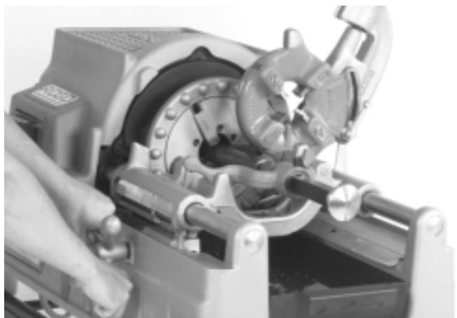
Figure 7 – Reaming with 341 Reamer
