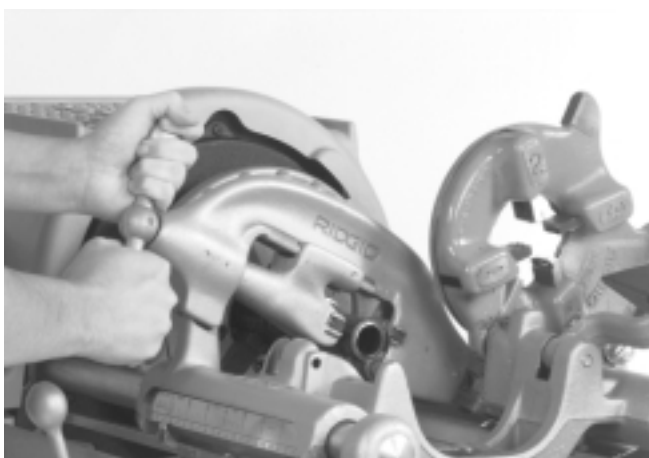
Figure 6 – Cutting Pipe with 820 Cutter
